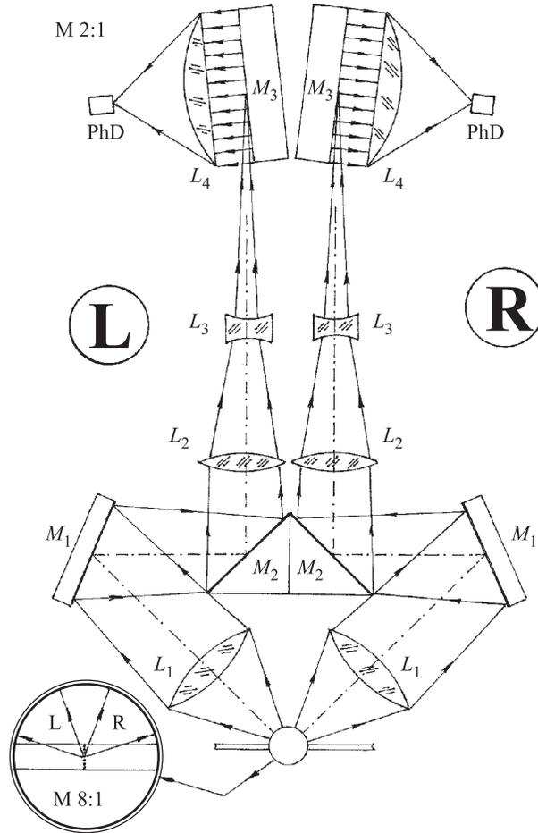
Fig. 4. Stereoscopic confocal scanner for the vertical particle tracks, provided with two confocal scanners on both sides of view (L and R):  $L_1$  — two main imaging lenses,  $L_2$  and  $L_3$  — two pair of Newton monocular lenses,  $L_4$  — two collecting lenses,  $M_1$  — two first-plane mirrors,  $M_2$  — two second-plane mirrors,  $M_3$  — two orthogonalization mirrors, PhD — two point-like photodiodes
