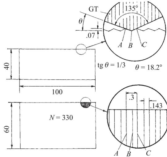
Fig. 3. Image orthogonalization system: GT — grooving tool; A, B and C are three points of the lamellar region, BC is the working part of the lamellar mirror. All dimensions — in mm
