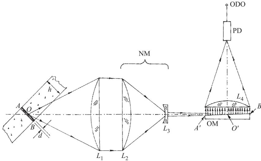
Fig. 2. The principal scheme of the confocal scanner for vertical particle tracks:  $L_1$  — main imaging lens,  $L_2$  and  $L_3$  — lenses of the Newton monocular,  $L_4$  — collecting lens, OM — orthogonalization mirror, PhD — point-like photodiode;  $A'$ ,  $O'$  and  $B'$  are the imaging points of  $A$ ,  $O$  and  $B$  points of the vertical particle track,  $d$  — width of the illuminating zone,  $\sim 2 \mu\text{m}$
