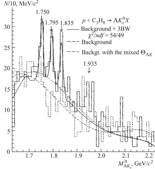
Fig. 3. Invariant mass distribution ( $\Lambda K_s^0$ ) with the bin size  $10 \text{ MeV}/c^2$  in the inclusive reaction  $p+C_3H_8$ . The solid curve is the sum of the experimental background by the first method (dot-dashed curve) and three Breit–Wigner resonance curves. The dashed histogram is the experimental background [25]
