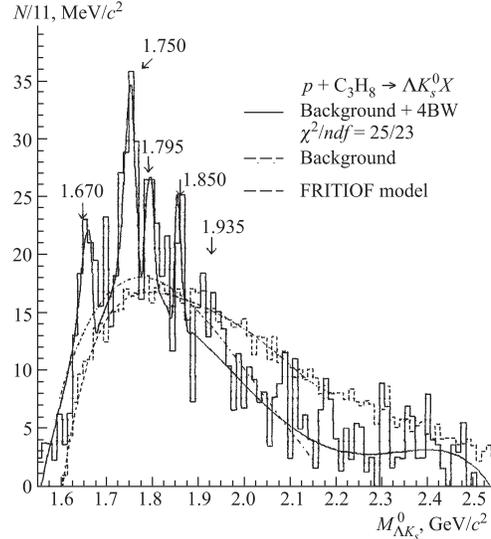
Fig. 5. Invariant mass distribution ( $\Lambda K_s^0 X$ ) with the bin size 11  $\text{MeV}/c^2$  in the inclusive reaction  $p+C_3H_8$ . The solid curve is the sum of the experimental background by the first method (dot-dashed curve) and four Breit–Wigner resonance curves. The dashed histogram is the simulation by FRITIOF model [26, 27]
