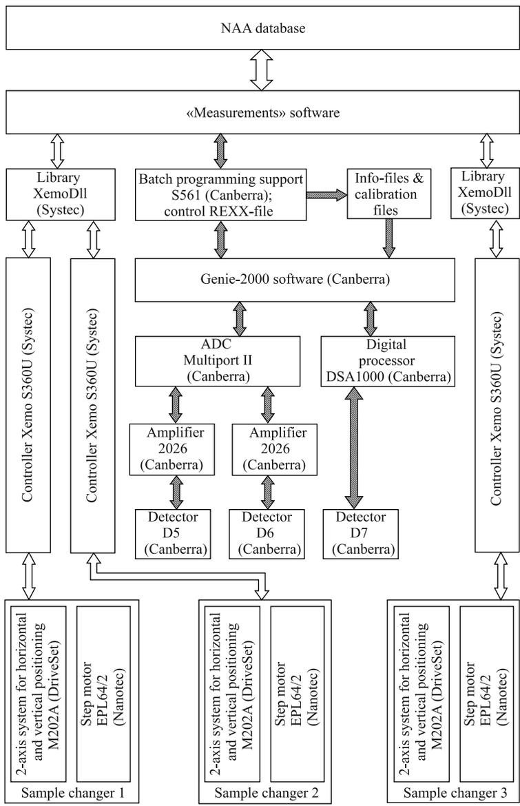
Fig. 1. The block diagram of automatic system of spectra measurement
