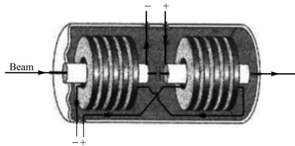
Fig. 8. Typical structure of a ferrite-loaded cavity [17]
