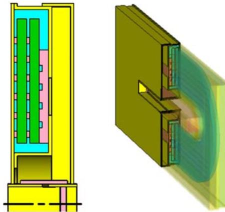
Fig. 13. Design of the MA cavity for the JINR FFAG (side view and axonometric projection)
