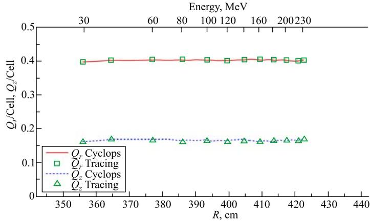
Fig. 6. Horizontal and vertical tune per cell
