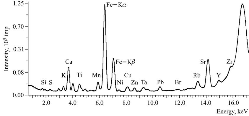
Fig. 1. XRF spectrum of coal sample
