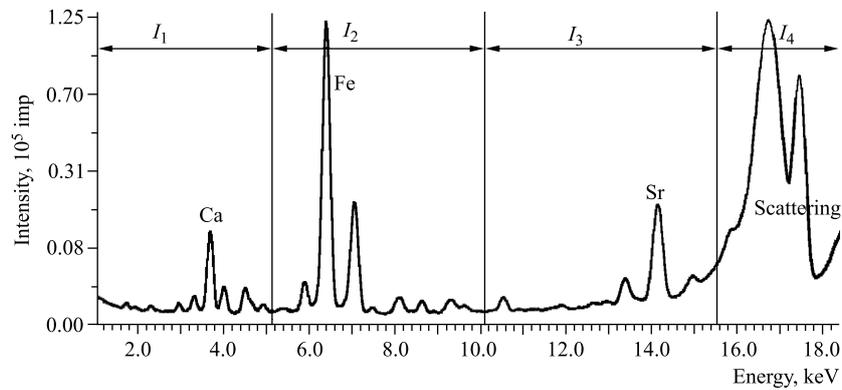
Fig. 2. Four divided X-ray spectrum for coal ash determination
