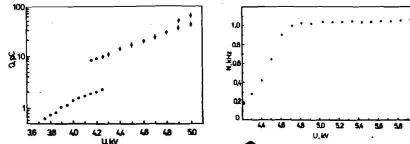
Fig. 3. Single rate curve of a detector of the hadron calorimeter prototype.
