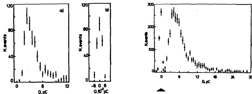
Fig. 9. Spectrum of signals from cosmic muons from a supertower:
