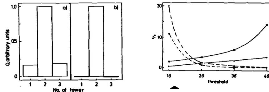
Fig. 11. Curves characterizing the efficiency of the muon trigger produced when the signals from two or three supertowers exceed the threshold expressed in terms of standard deviations of the noise signal: full lines-inefficiency of the trigger (relative to the external trigger), dotted lines- relative number of accidental triggers; points-data for two supertowers, crosses- for three supertowers.
