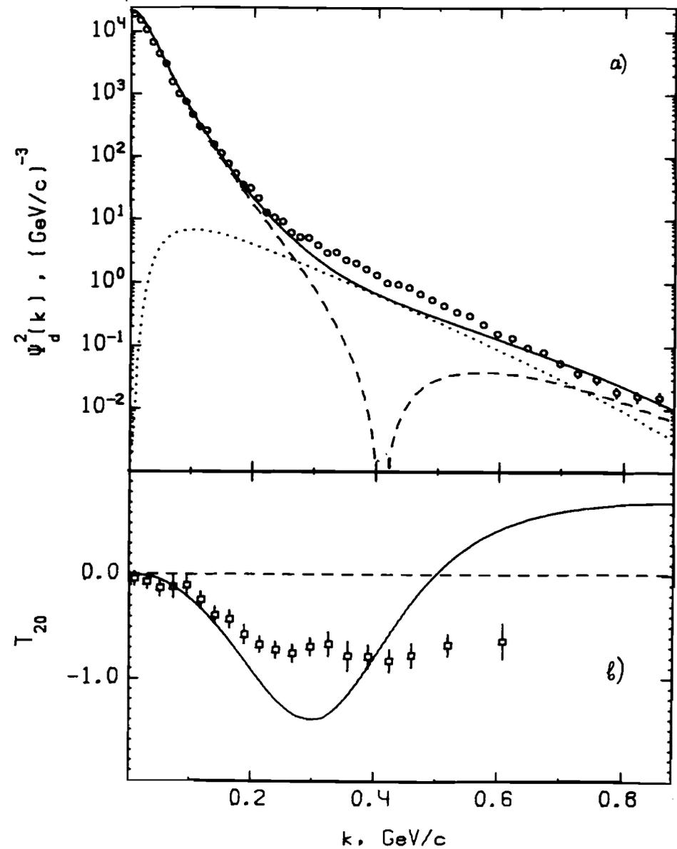
Fig.2. a) The NMDD versus the interval momentum  $k$ ; solid line -  $\psi_d^2(k)$ , dashed line -  $u^2(k)$ , dotted line -  $w^2(k)$ ,  $\circ$  - DUBNA (our data). b) The tensor analyzing power  $T_{20}$  versus  $k$ ;  $\square$  - DUBNA (our data), solid line - impulse approximation for the Paris NN - potential.
