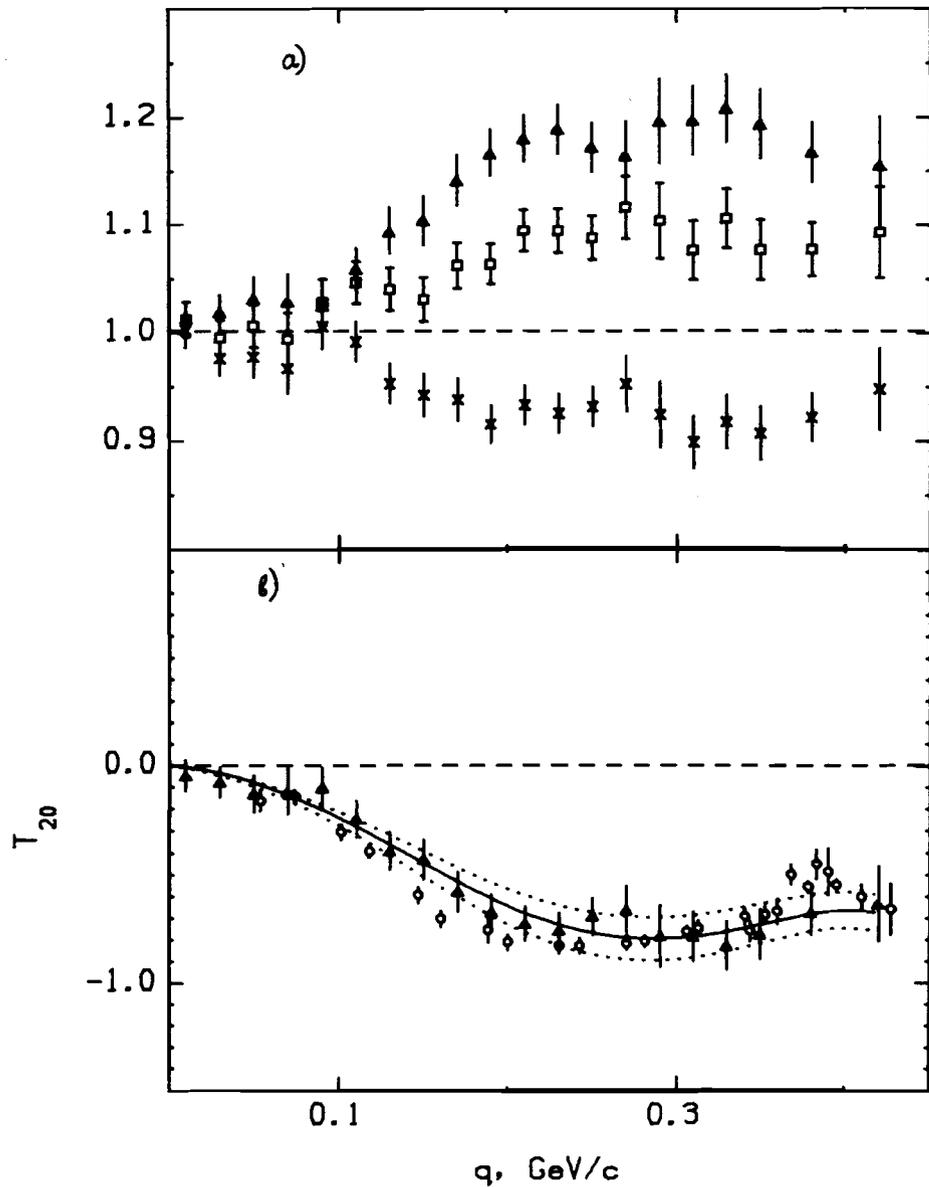
Fig.1. a) The cross section ratios versus the proton momentum  $q$  in the deuteron rest frame;  $\square - \sigma(+)/\sigma$ ,  $\times - \sigma(-)/\sigma$ ,  $- \sigma(+)/\sigma(-)$ . b) The experimentally obtained tensor analyzing power  $T_{20}$  of the  $^{12}\text{C}(d,p)$  reaction versus  $q$ ;  $\blacktriangle$  - DUBNA (our data),  $\circ$  - SACLAY (ref. <sup>12'</sup>), solid and dotted lines - see the text.
