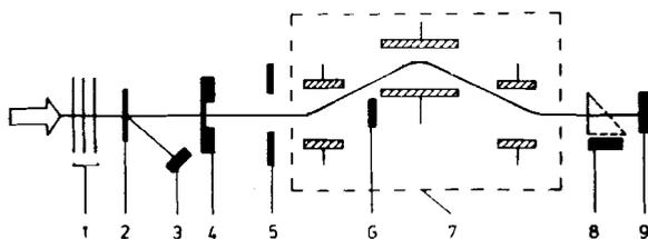
Fig.1. A schematic view of the experimental set-up. 1 - degraders, 2 - Au-scatterer, 3 - detector designed to determine the beam energy, 4 - rotating target, 5 - input diaphragm, 6 - Faraday cup, 7 - separator "VASSILISSA", 8 - time-of-flight detectors, Si(Au)-detector.
