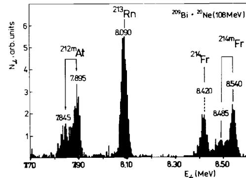
Fig.3. The alpha-spectrum from evaporation residues produced in the  $^{209}\text{Bi} + ^{20}\text{Ne}$  reaction at a beam energy of 108 MeV.
