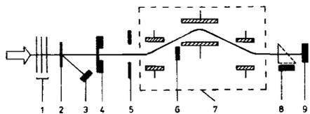
Fig.1. Schematic view of the "Vassilissa" facility. 1 - absorbers, 2 - Au scatterer, 3 - detector to determine the energy of the scattered ions, 4 - target, 5 - input diaphragm, 6 - Faraday cup, 7 - separator Vassilissa, 8 - time of flight detectors, 9 - Si(Au) detectors.
