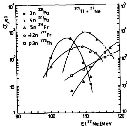
Fig.6. The differential cross-section of the  $^{205}\text{Tl} + ^{22}\text{Ne}$  reaction products. The left scale stands for  $\alpha, 2n$ , the right scale is for the xn and pxn evaporation channels.
