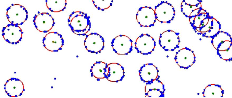
Fig. 1. Part of one typical event in the CBM RICH detector: RICH hits, found RICH rings
