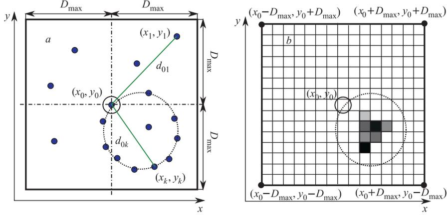
Fig. 2. *a)* Preliminary local hit selection in a region defined by the maximum ring diameter plus a safety margin. *b)* Schematic view of the 2D histogram of ring centers
