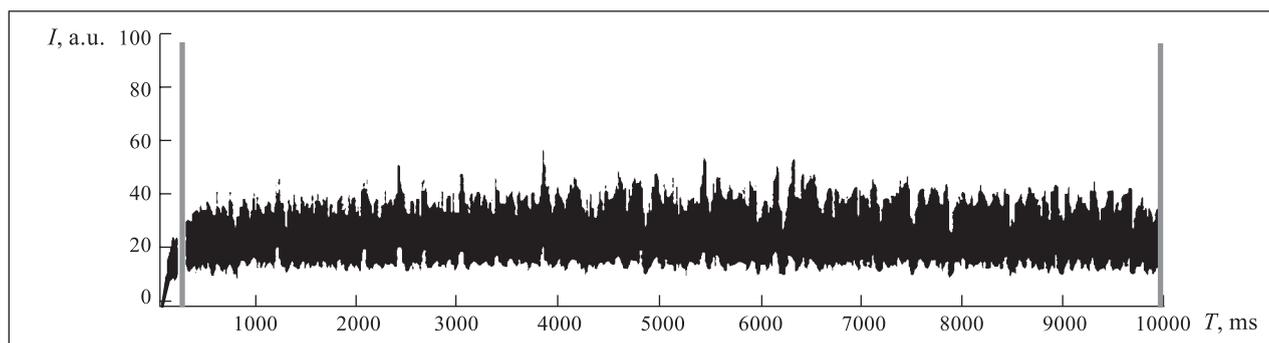
Fig. 2. A pulse duration of an extracted beam
