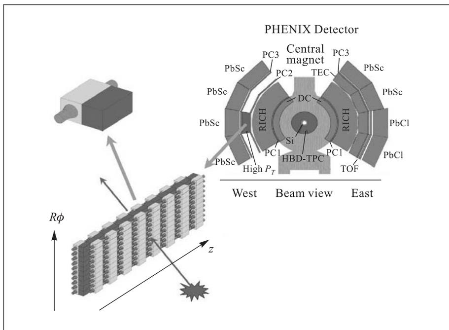
Fig. 7. The layout of the aerogel subsystem installed at PHENIX
