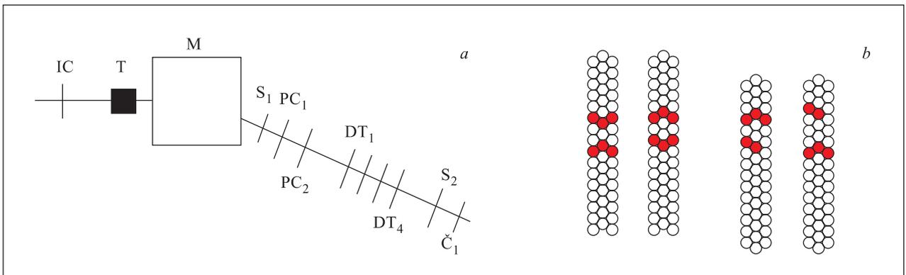
Fig. 4. a) The scheme of the STRELA set-up. b) Samples of events with two protons in the drift tubes
