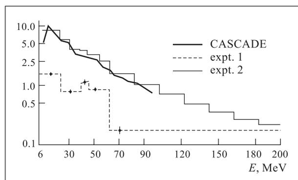
Fig. 12. Experimental and theoretical neutron spectra on the moderator surface of the GAMMA-2 set-up. Here «expt. 1» stands for our measurement and method, «expt. 2» for other method applied to our data, CASCADE — calculations made by Prof. V. S. Barashenkov
